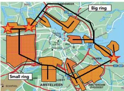
figure 4 Future scenario : single heat provider and closed network
